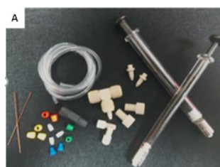
Figure A. Set of tubing, syringes and connecting used for millifluidics device design. ©Chloe Amine
