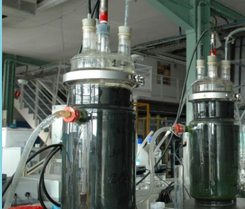
Lab-scale anaerobic biogas reactor. ©LBE - INRAE
