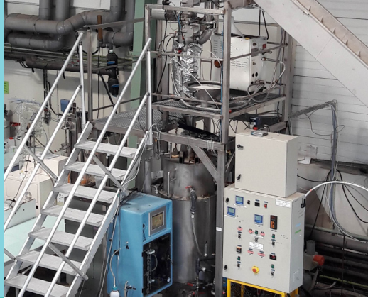
INRAE-LBE pilot-scale two-step organic-route hydrogen and methane production unit. ©INRAE
